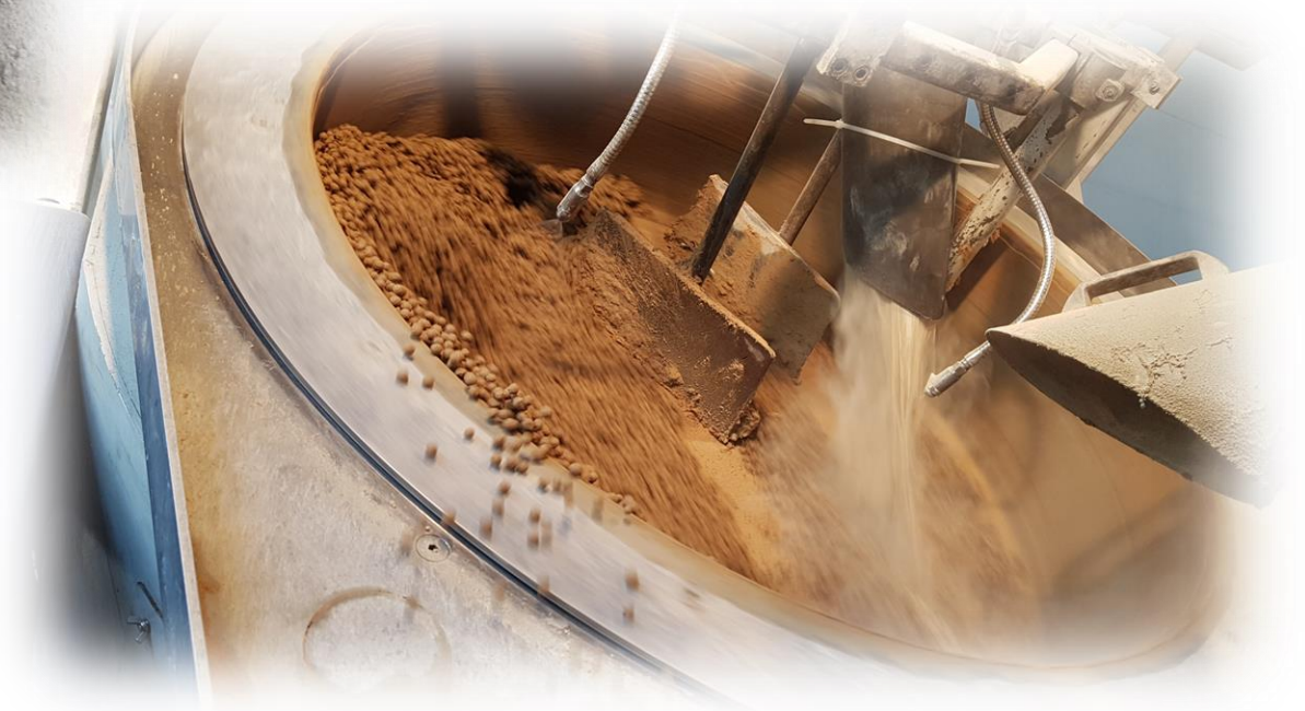
Agglomeration in the pelletizing disc
